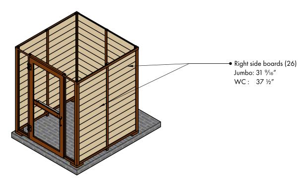
On the front, slide in the plastic lumber from the top in the same way with groove down, tongue up, and textured side out. Remove the aluminum angle and install the plastic lumber on the door last. Note decal
