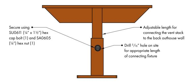
Install the connecting fixture to the back of the outhouse, as shown below. With the John Outhouse, it may be preferable to connect the fixture to the roof slots instead of the back wall.
