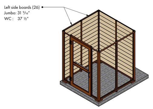
On the right side, slide in the plastic lumber from the top in the same way with groove down, tongue up, and textured side out.
