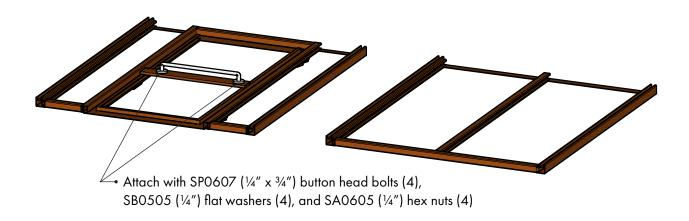
Attach the four corner feet to the bottom of the front and back panels.
