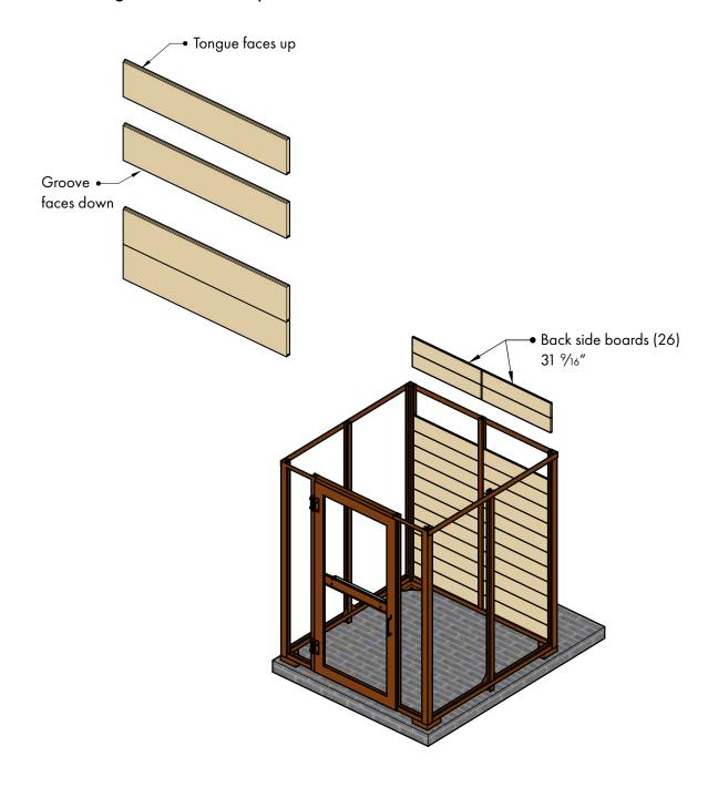
On the left side, slide in the plastic lumber from the top in the same way with groove down, tongue up, and textured side out.
