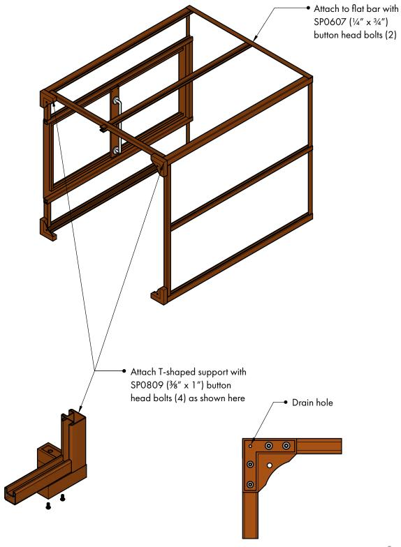
Turn over the frame and attach the remaining side supports as in steps 3 and 4. First attach the upper flat bar. Then loosely attach the top of the T-shaped support to it before attaching the bottom to the corner feet. Tighten all bolts when square.
