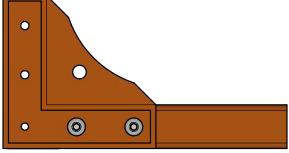
Stand the panels on edge with the channels facing each other as shown. Attach the flat bar side support to the top of the panels on one side of the frame.
