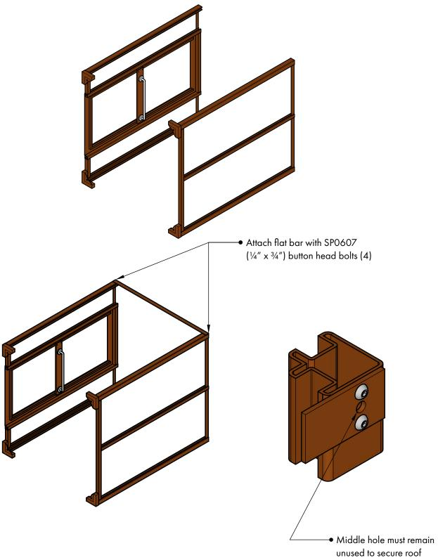
On the same side of the frame, loosely attach the T-shaped side support to the upper flat bar before attaching the lower part of the T-shaped support to the corner feet. Tighten all bolts at the end.
