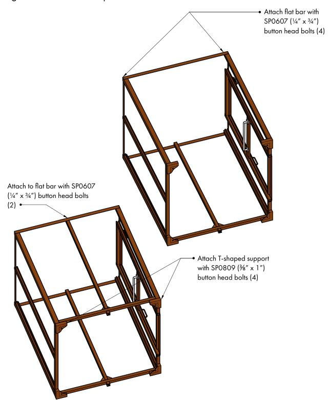
Stand up the outhouse frame in the location to be secured. Level and square the frame before appropriately securing it to the pad or ground with fasteners supplied by the installer. Spacers under the corner blocks may be required. Ensure the door moves freely and closes properly.
