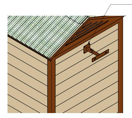
Position connecting fixture and drill four <sup>5</sup>/16" holes through the plastic lumber on the back wall. Attach with SJ0614 (1/4" x 2 1/4") carriage bolts (4) from the inside and SB0505 (1/4") flat washers and SA0605 (1/4") hex nuts (4 of each) on the outside.
