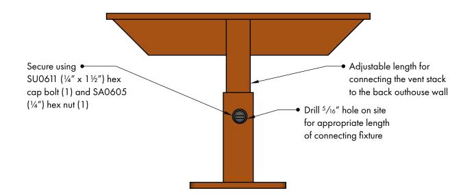
15 Install the connecting fixture to the back of the outhouse, as shown below. With the John Outhouse, it may be preferable to connect the fixture to the roof slots instead of the back wall.
