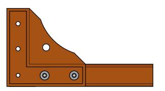
Stand the panels on edge with the channels facing each other as shown. Attach the flat bar side support to the top of the panels on one side of the frame.
